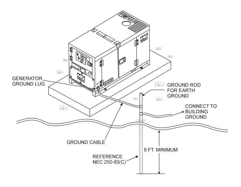
**Figure 4. Typical Generator Grounding Application**
